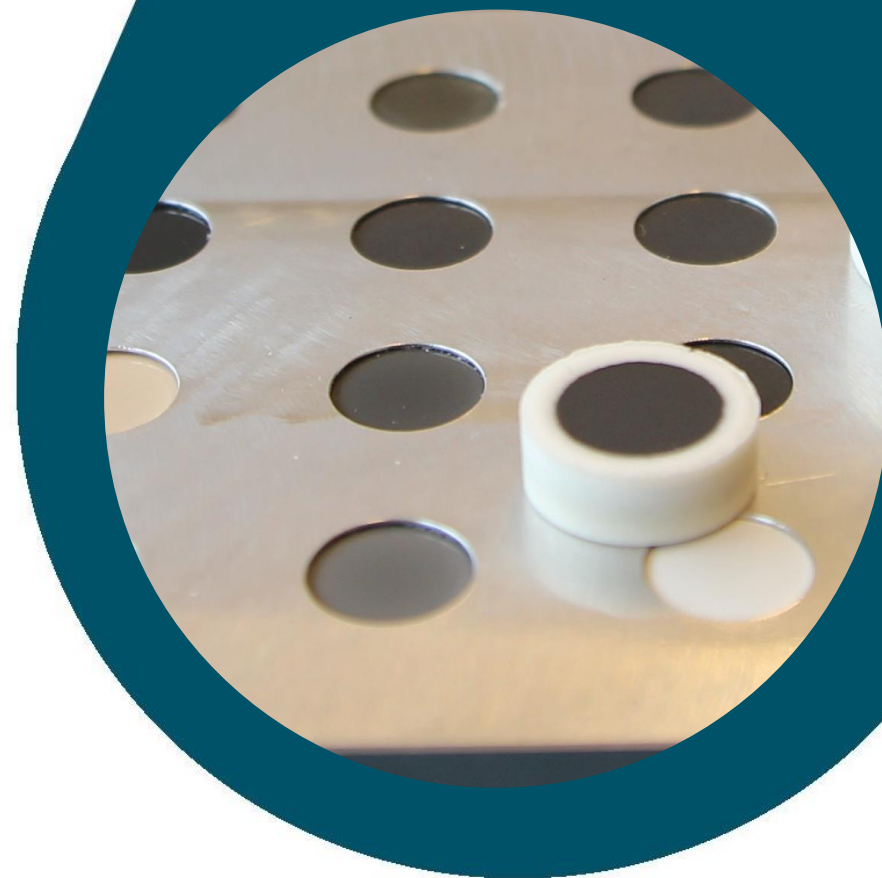
Measurement Setup inside M4 Tornado similar. Pellets inside CNC-milled aluminium Mount
