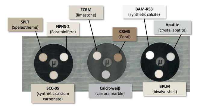
Elemental homogeneity tests using larger laser spot size: 80 µm microanalysis? mapping?
