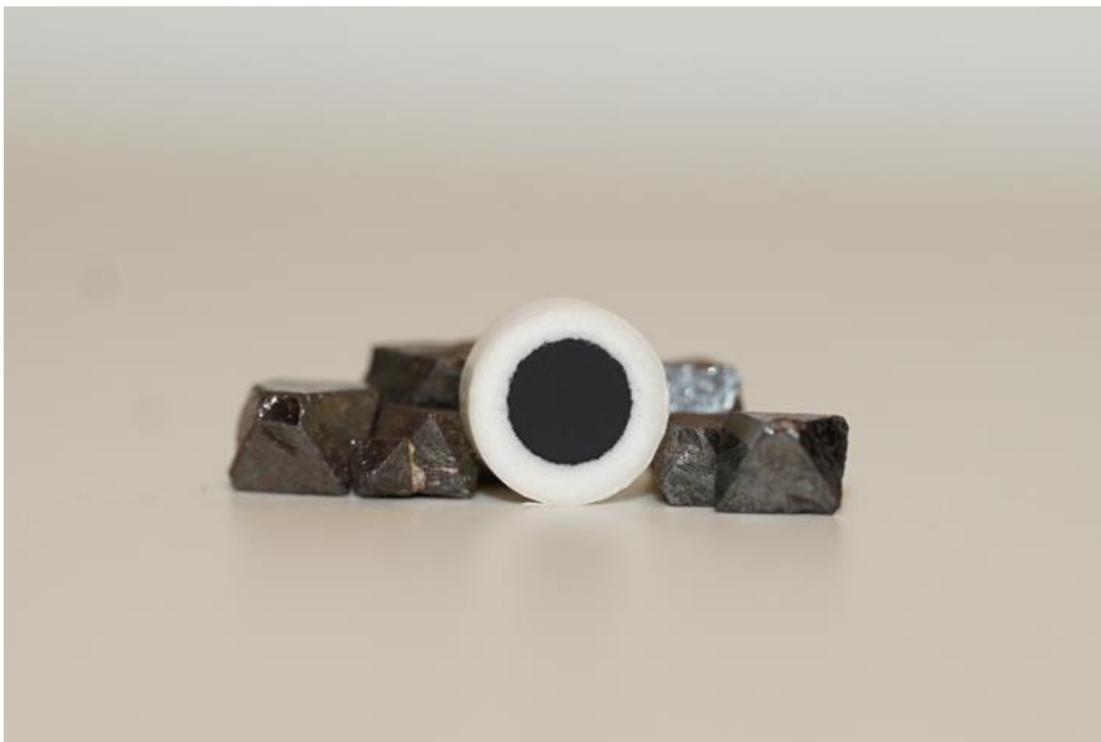
Fig. 1 Photograph of magnetite crystals and the resulting Nano-Pellet.
