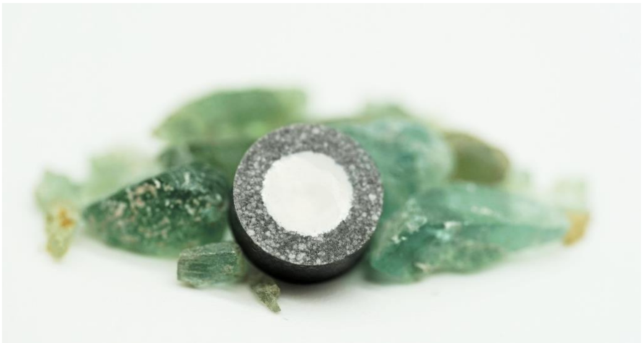
Fig. 1 Photograph of the apatite crystals and a Nano-Pellet made from them.
