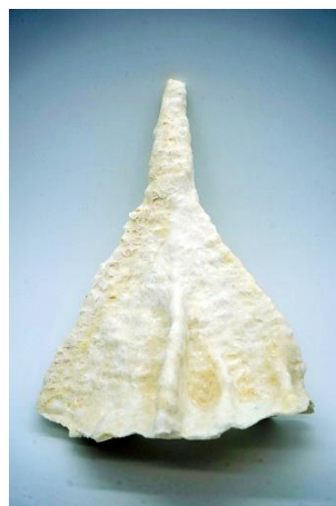
Fig. 1 Photograph of a speleothem found on a concrete ceiling in the Berlin Zoo.
