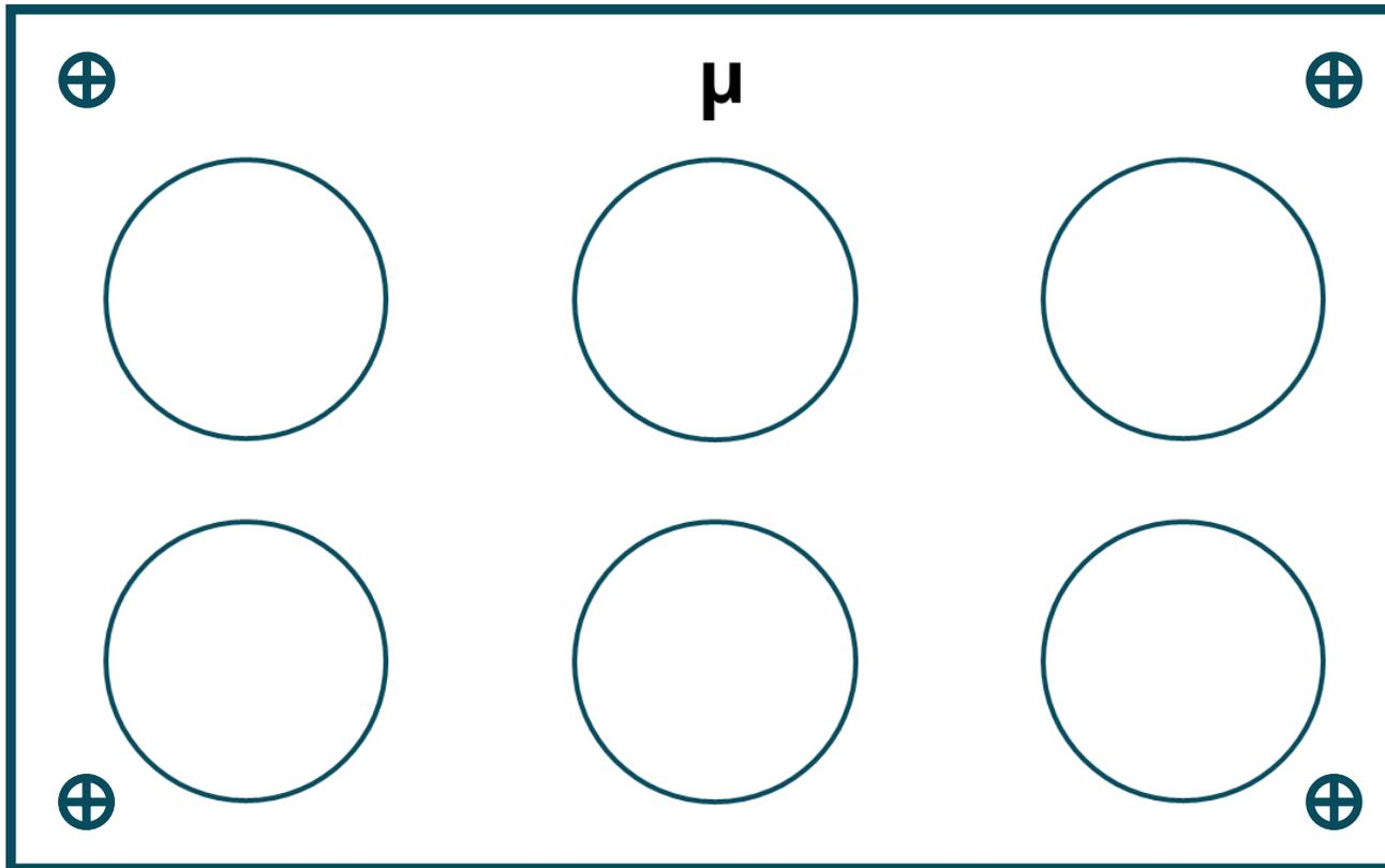
Mount made of aircraft grade aluminium (7075) and coated with Diamond-Like-Carbon (DLC)© for holding up to 6 x 10 mm diameter nano-pellets. Laser-engraved to facilitate stage alignment.
